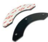
HE-XBP-MPPL Custom Steel Permanent Mounting Kit with (2) steel plates, powder-coated for rust protection & (6) holes to secure to beacon. 3M VHB adhesive on base of plates for mounting to Non-metallic surfaces.
